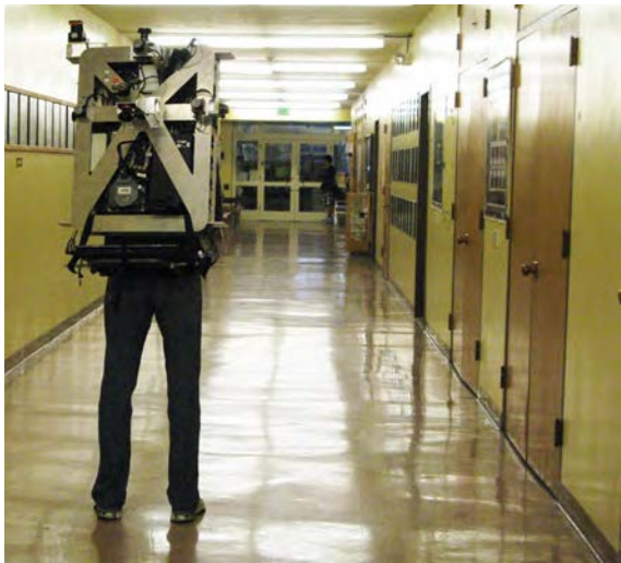
Figure 15-12: An example of indoor, three-dimensional data acquisition and organization. Image and LiDAR data collected with a backpack system (top) provide three-dimensional reconstructions of indoor environments (middle). These may be combined, maintaining accurate absolute position, to reconstruct connected building interiors (bottom). While currently an active research area, progress is apparent in applications, and will accelerate as data collection, storage, processing, and analysis hurdles are overcome, and as standards are established for data storage and access (courtesy Avidesh Zakhor, U.C. Berkeley Video and Image Processing Lab).
