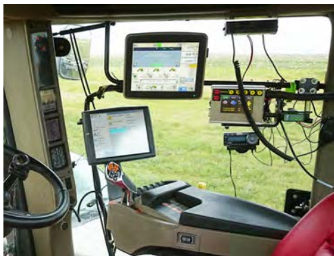
Figure 5-28: Line features may be field digitized via GPS, as in this example of a GIS/GPS system mounted in a tractor. Data display and digitizing software are used to record coordinates collected by a GPS receiver (above). An antenna placed on a pole or rack (right) reduces obstruction (courtesy Jake Leguee, left, and G. Johnson, Ducks Unlimited, right).
