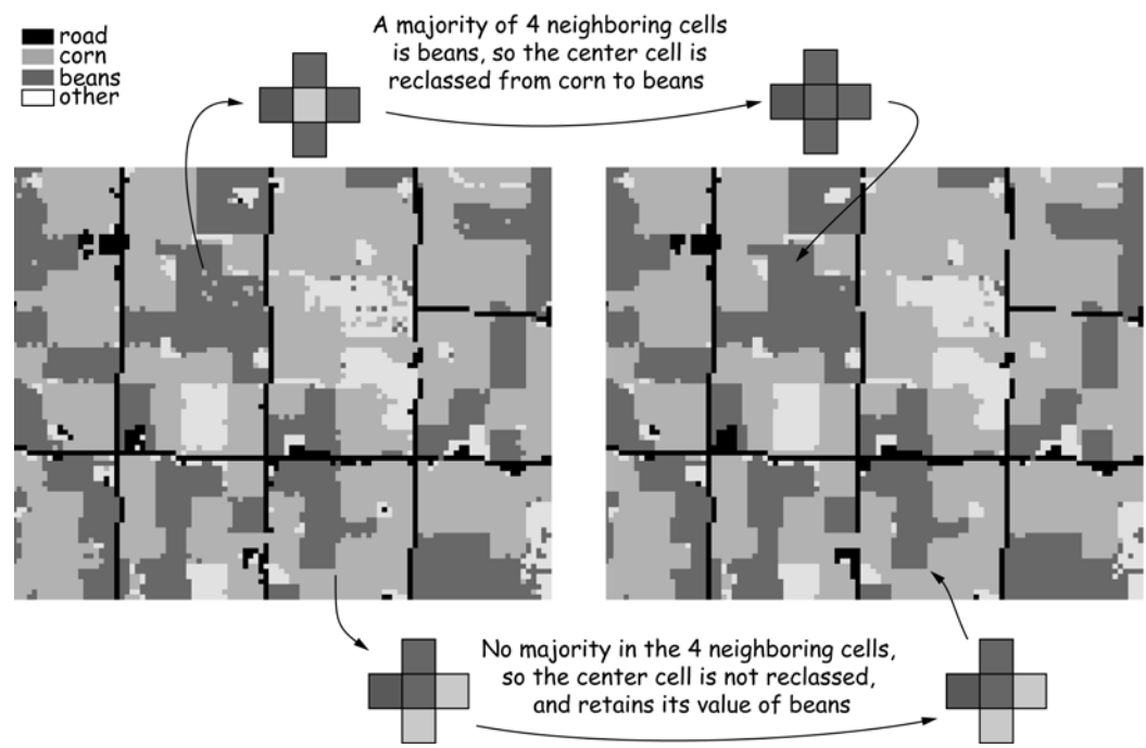
Figure 10-17: An example of a majority filter applied to a raster data layer from a classified satellite image. Many isolated cells are converted to the category of the dominant surrounding class.
