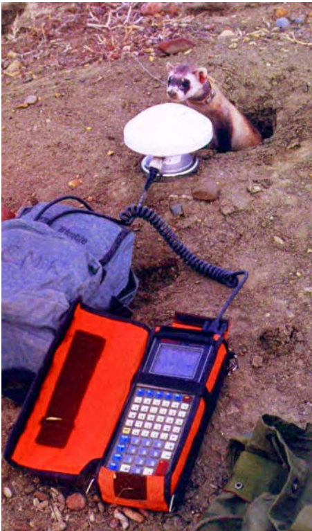
Figure 1-12: Specialized equipment is used to collect spatial data. Here a burrow location is recorded using a GPS receiver, as an interested black footed ferret looks on (courtesy Randy Matchett, USFWS).
