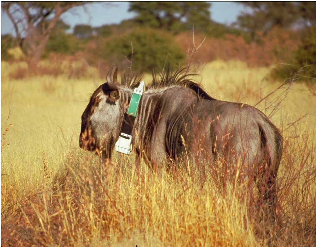
Figure 5-37: A wildebeest fit with a GNSS tracking collar. The antenna is visible as the white patch on top of the collar, and the power supply and data logging housing is visible at the bottom of the collar. Animal position is tracked day and night, yielding substantially improved information on animal activity and habitat use. (Courtesy Gordon T. Carl, Lotek Wireless Inc.)
