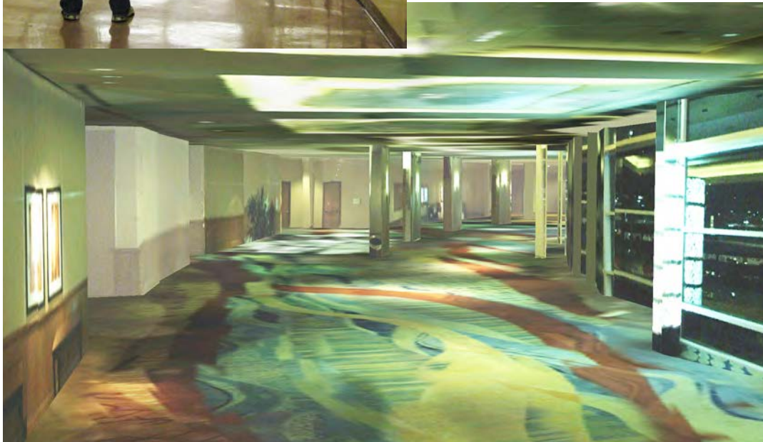
Figure 15-12: An example of indoor, three-dimensional data acquisition and organization. Image and LiDAR data collected with a backpack system (top) provide three-dimensional reconstructions of indoor environments (middle). These may be combined, maintaining accurate absolute position, to reconstruct connected building interiors (bottom). While currently an active research area, progress is apparent in applications, and will accelerate as data collection, storage, processing, and analysis hurdles are overcome, and as standards are established for data storage and access (courtesy Avidesh Zakhor, U.C. Berkeley Video and Image Processing Lab).
