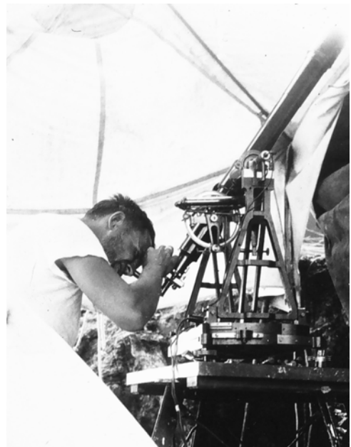
Figure 3-12: Astronomical observations were used in early geodetic surveys to measure datum locations (courtesy NOAA).
