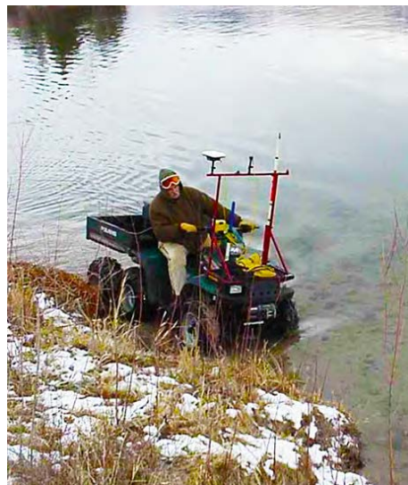
Figure 5-28: Line features may be field digitized via GPS, as in this example of a GIS/GPS system mounted in a tractor. Data display and digitizing software are used to record coordinates collected by a GPS receiver (above). An antenna placed on a pole or rack (right) reduces obstruction (courtesy Jake Leguee, left, and G. Johnson, Ducks Unlimited, right).
