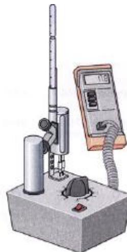
An instrument used to measure melting point.
